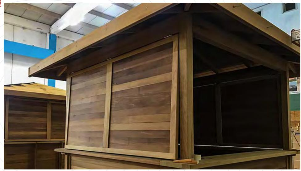
Towel cabanas / Towel Dispenser Units with movable mechanisms and retractable doors were manufactured from extra quality solid iroko wood for One&Only Portonovi Resort in Montenegro. For the project, the architectural designs of which were made abroad, the cabanas were prepared from imported structural wood materials, and were manufactured in the company's factory in Yalova. The assembly and installation were carried out at the facility in Montenegro.
